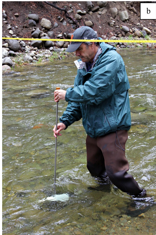
Figure 5-2. Scott Hackley of TERC collecting samples at Blackwood Creek. (a) Stretching a tape across the creek for EWI sampling; (b) Collecting a chemistry sample with the DH81 sampler; (c) Pouring the sample into the churn splitter. Photos by Jim Markle ( http://jimmarkle.smugmug.com/ ).
