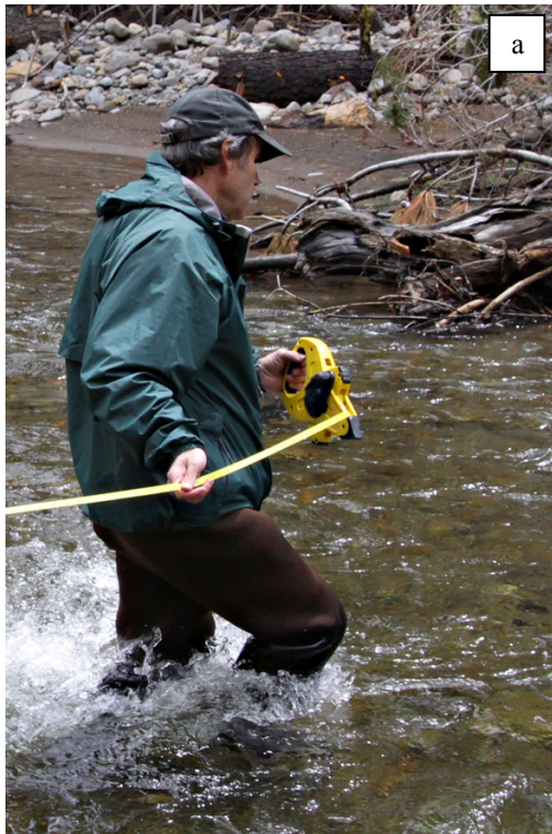
Figure 5-2. Scott Hackley of TERC collecting samples at Blackwood Creek. (a) Stretching a tape across the creek for EWI sampling; (b) Collecting a chemistry sample with the DH81 sampler; (c) Pouring the sample into the churn splitter. Photos by Jim Markle ( http://jimmarkle.smugmug.com/ ).
