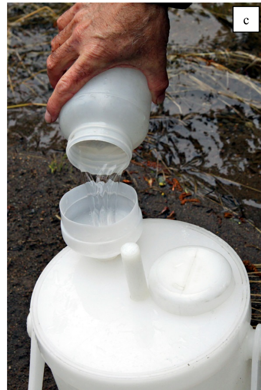
Figure 5-2. Scott Hackley of TERC collecting samples at Blackwood Creek. (a) Stretching a tape across the creek for EWI sampling; (b) Collecting a chemistry sample with the DH81 sampler; (c) Pouring the sample into the churn splitter. Photos by Jim Markle ( http://jimmarkle.smugmug.com/ ).
