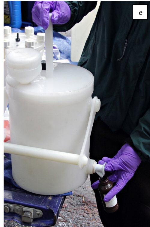
Figure 5-2. Scott Hackley of TERC collecting samples at Blackwood Creek. (d) Filtering a sample for analysis of dissolved constituents; (e) Collecting an unfiltered sample from the churn splitter for TP and TKN; (f) Labeling a sample bottle. Photos by Jim Markle ( http://jimmarkle.smugmug.com/ ).
